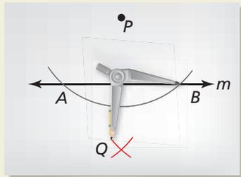
**Draw intersecting arcs** Draw an arc with center  $A$ . Using the same radius, draw an arc with center  $B$ . Label the intersection of the arcs  $Q$ .
