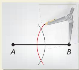
**Draw a second arc** Keep the same compass setting. Place the compass at  $B$ . Draw an arc. It should intersect the other arc at two points.
