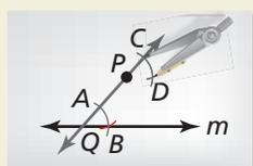
**Copy angle** Draw an arc with radius  $AB$  and center  $A$ . Using the same compass setting, draw an arc with center  $C$ . Label the intersection  $D$ .
