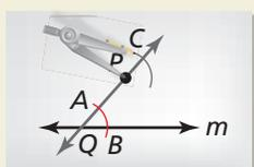
**Draw arcs** Draw an arc with center  $Q$  that crosses  $\overline{QP}$  and line  $m$ . Label points  $A$  and  $B$ . Using the same compass setting, draw an arc with center  $P$ . Label point  $C$ .
